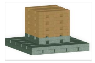
Figure 7. Wood block Foundation – Proposed Development Approach
