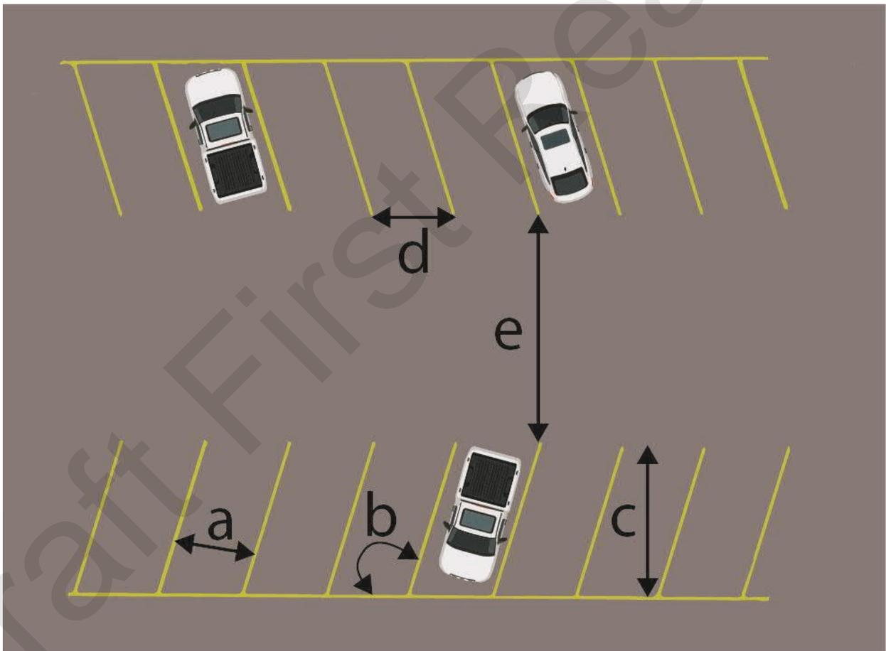
6.11.7 Notwithstanding **Subsection 6.11.6**, if a parking stall is adjacent to a permanent structure including but not limited to buildings or pillars, the parking stall shall have a minimum width of 3.00 m (9.84 feet).
